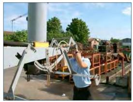
Tie the filling hole of the big bag with the appropriate rope.
