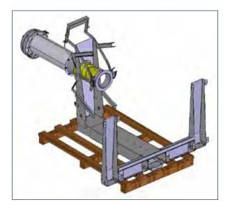
7) Fasten the filter leaning base to the appropriate bracket tightening all the bolts properly.
