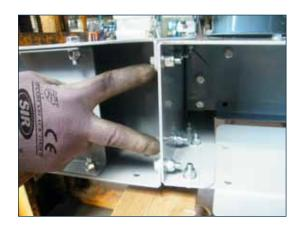
4) Position the L crosspiece as illustrated in the following picture, paying attention to match the holes on the crosspiece with the suitable crews; then fasten the crosspiece with the supplied screws.
