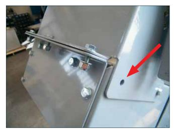
By means of a suitable lifting device, lift the EASYFILL<sup>TM</sup> up to its working position, hooking the two lifting lugs to the sides of the filter leaning base, rotating it around at about  $90^{\circ}$ .
