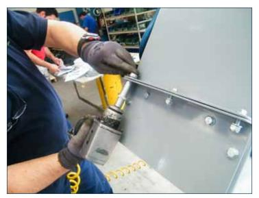
Insert and fasten the two bolts on the sides of the filter leaning base.
