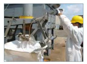
When starting the system for the first time, check that the height of the big-bag is appropriate in such a way as to prevent the weight of the big bag leans against the EASYFILL<sup>™</sup> structure during the filling process.
