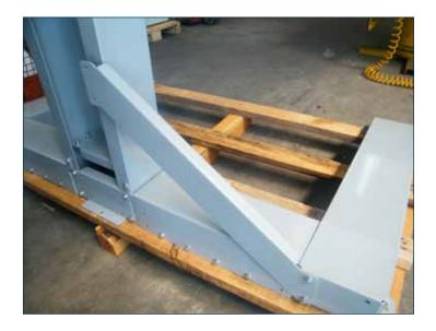
Then, assemble the two opening arms of the big-bag according to the direction of the hooks, as shown in the following picture.
