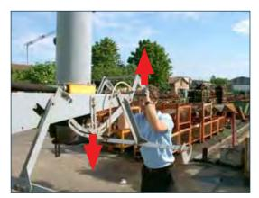
Insert the filling hole of the big-bag into the sealing collar as shown in the following picture.
